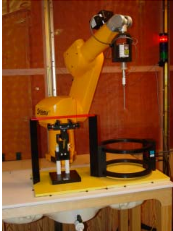
Figure 5.2a T-Coil setup with Helmholtz Coil
