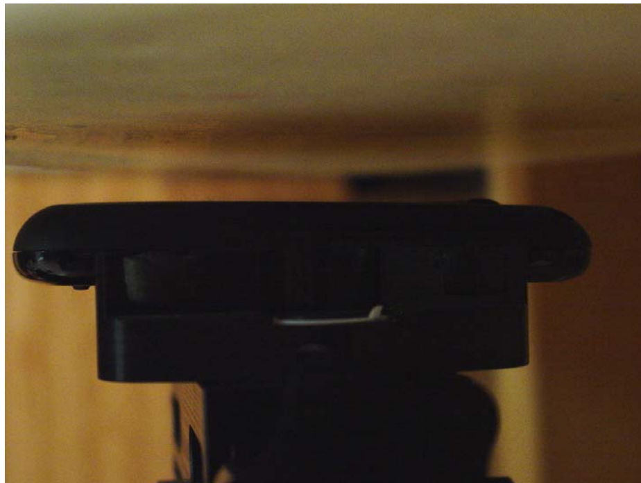
Figure 9E.3 Body SAR setup (15mm Air Separation)
