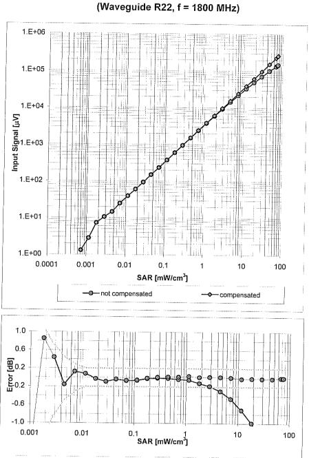
Dynamic Range f(SAR<sub>head</sub>) (Waveguide R22, f = 1800 MHz)
