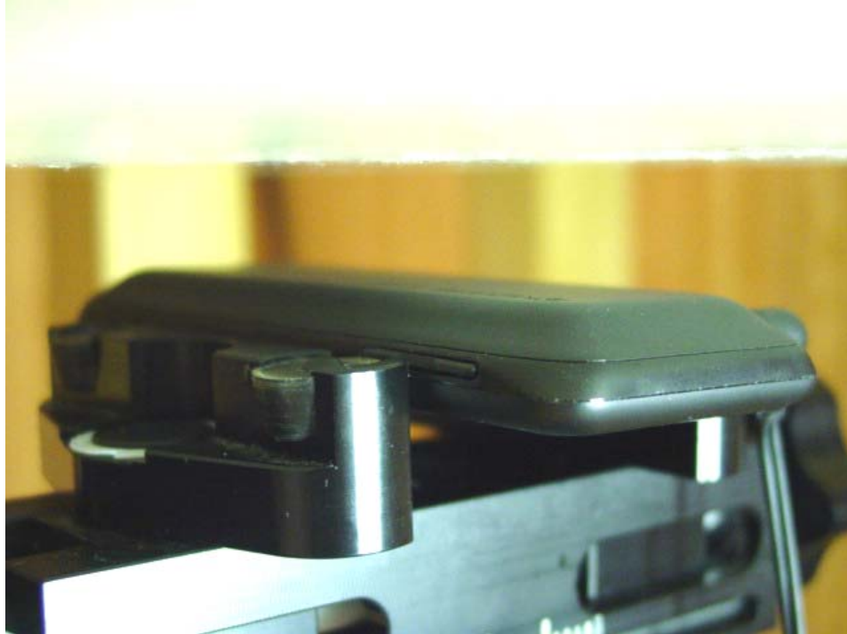
Figure 9E.3 Body SAR setup (15mm Air Separation)
