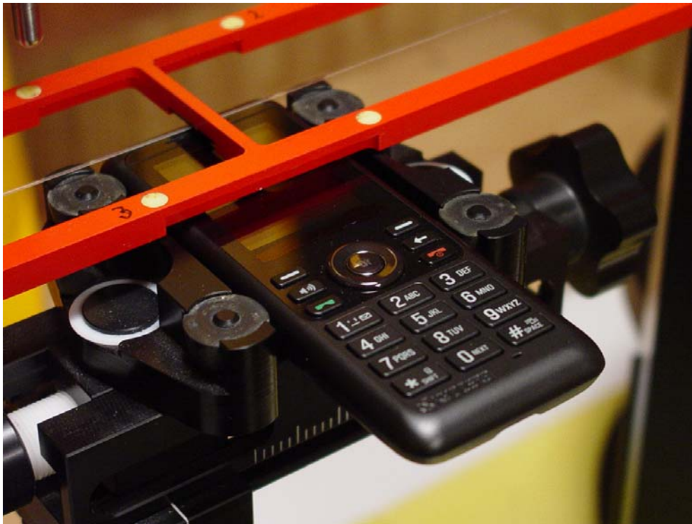
Figure 1a - HAC T-Coil Test Setup
