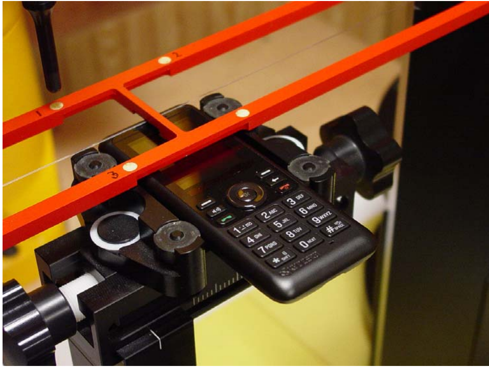
Figure 1a – HAC-RF Test Setup
