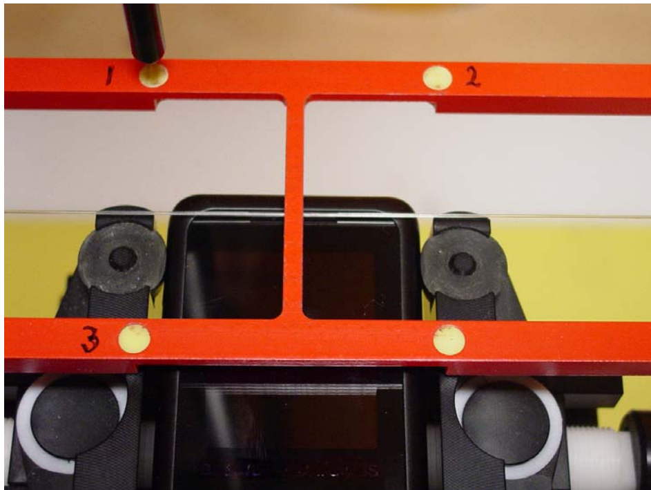
Figure 1b – HAC-RF Test Setup
