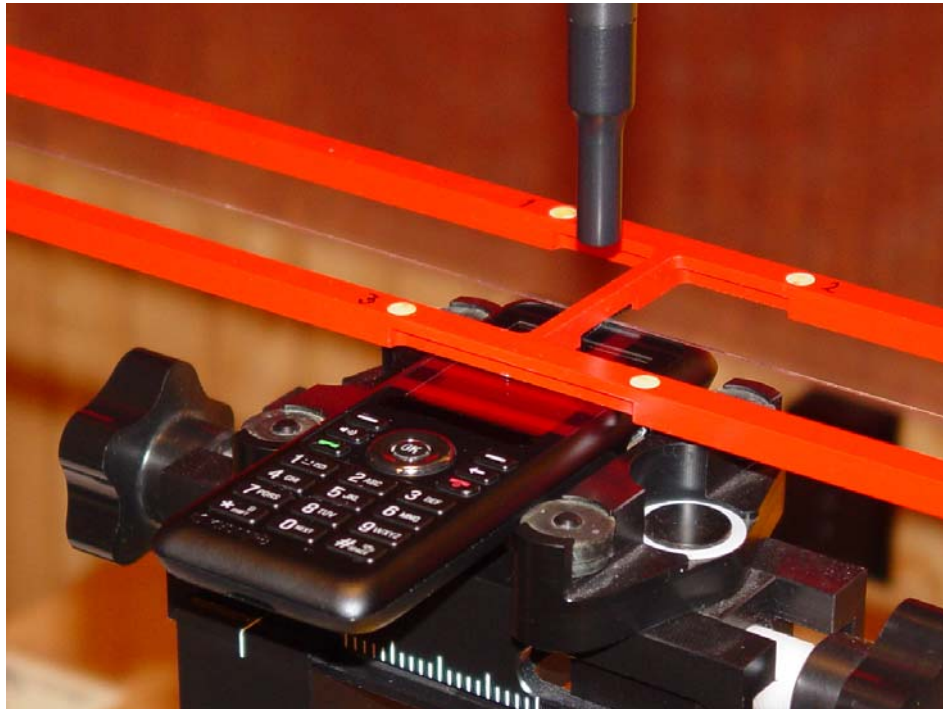
Figure 1a – HAC-RF Test Setup
