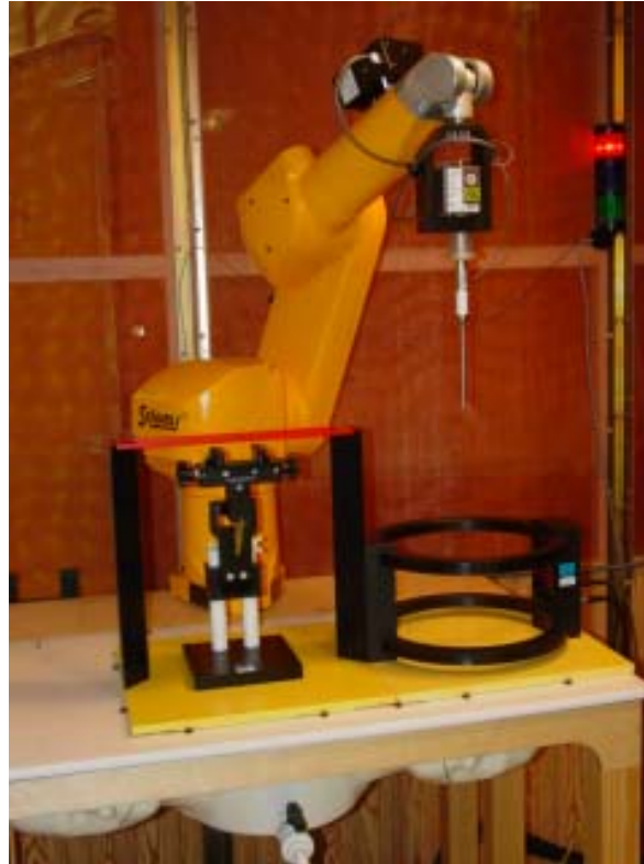
Figure 5.2a T-Coil setup with Helmholtz Coil
