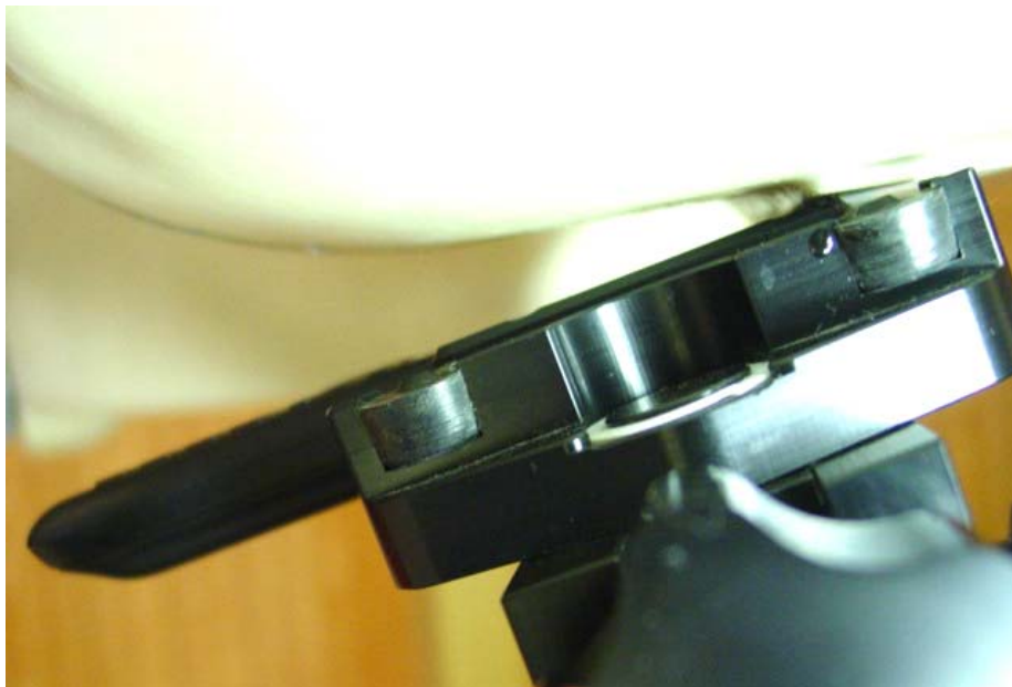
Figure 9E.1 Phone against the head (Left cheek position)
