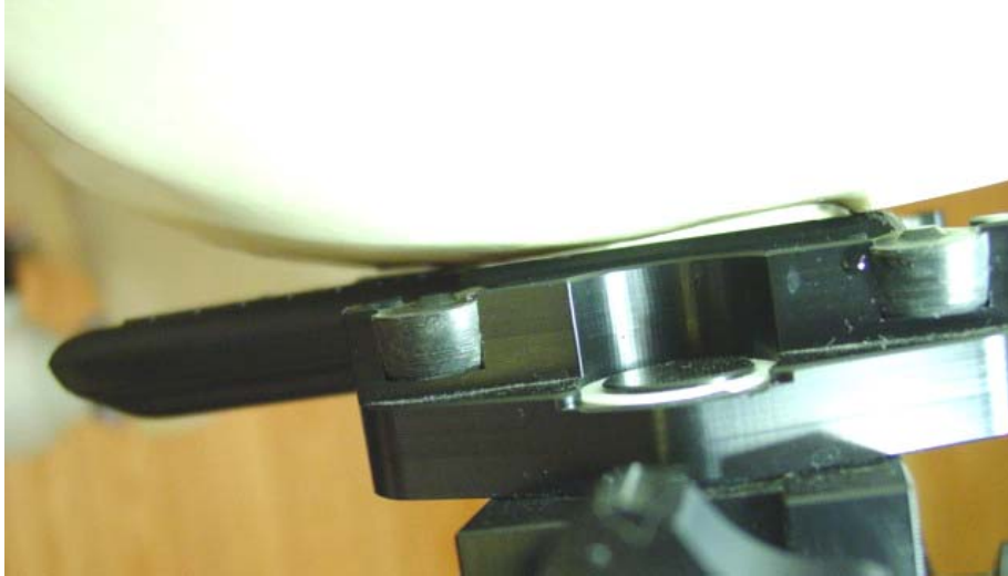
Figure 9E.1 Phone against the head (Left cheek position)
