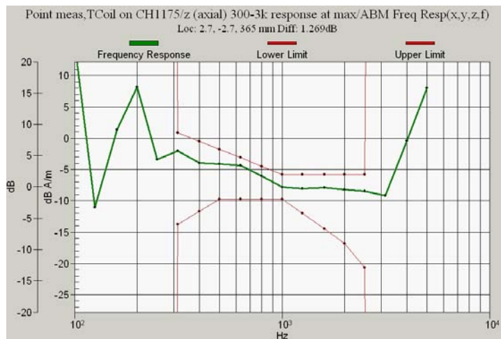
Figure 10.2i CDMA 1900 Channel 1175 Frequency Response
