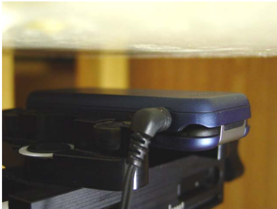
Figure 9E.3 Body SAR Phone setup Flip Closed (15mm Air Separation)
