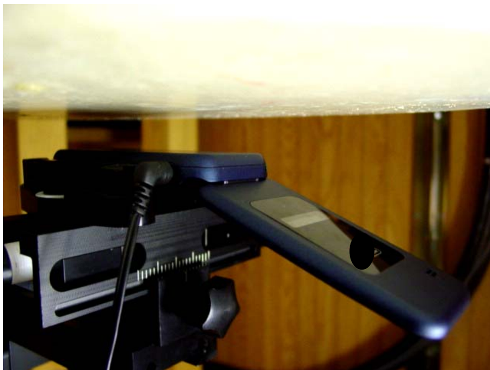
Figure 9E.4 Body SAR Phone setup Flip Opened (15 mm Air Separation)
