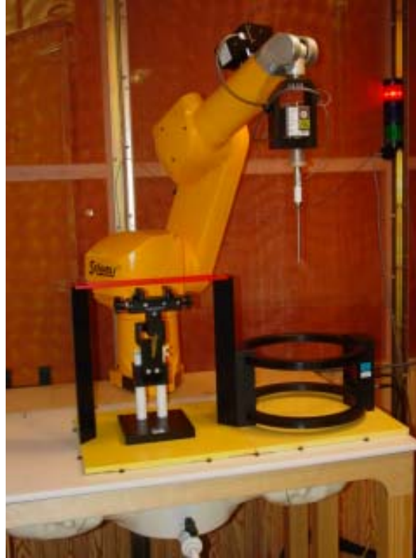
Figure 5.2a T-Coil setup with Helmholtz Coil
