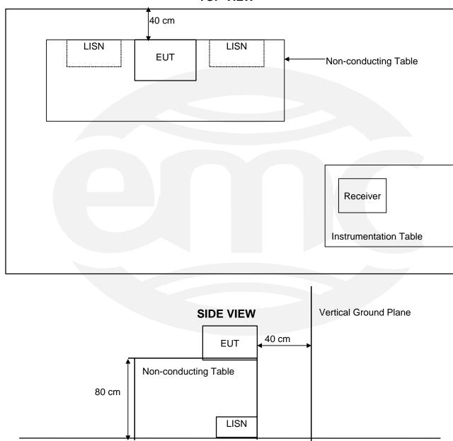
Other Measurements: 2 meters from top of EUT to ceiling 80 cm from closest part of EUT to the LISN
