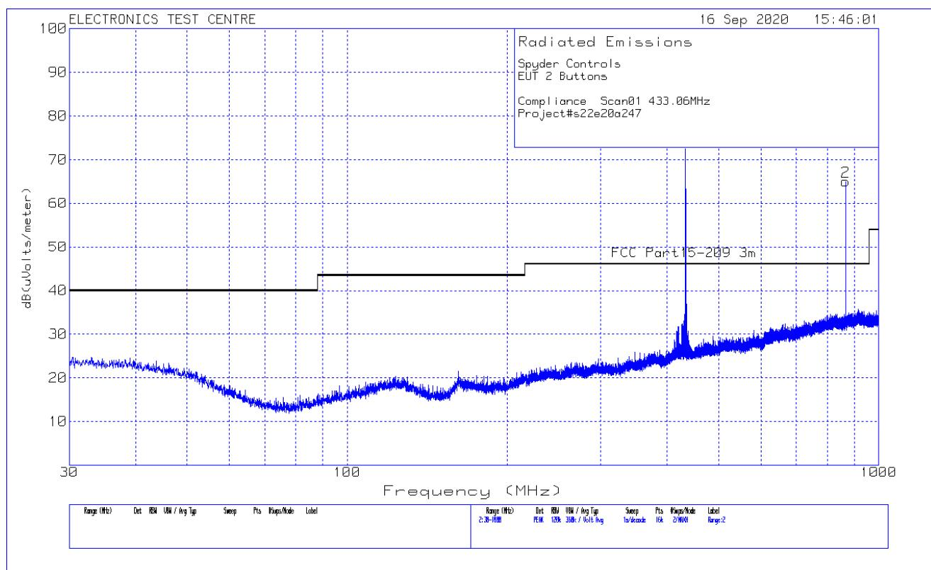
Plot of Radiated Emissions: Horizontal polarization [Tx@433.06 MHz](#)
