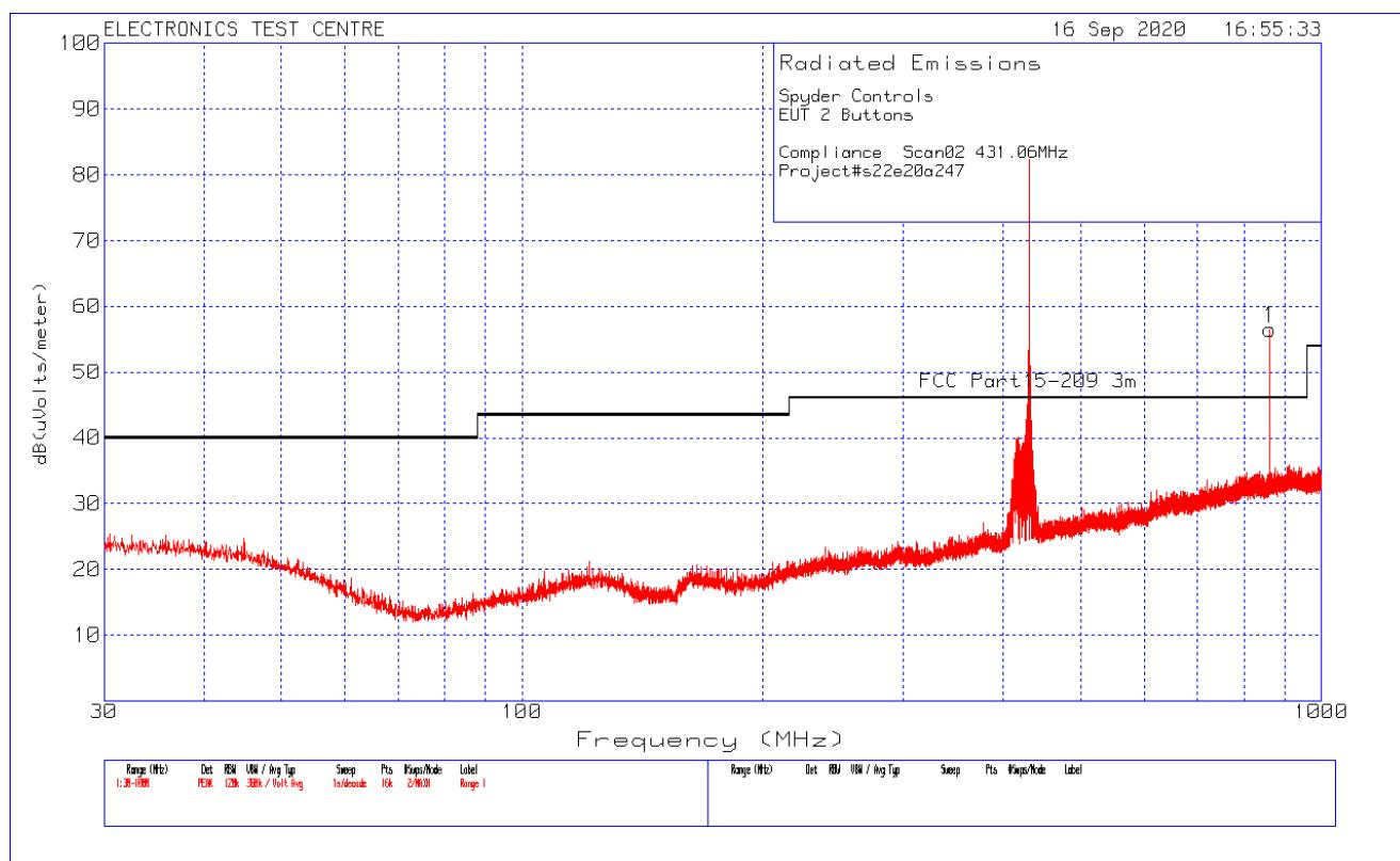
Plot of Radiated Emissions: Vertical polarization [TX@431.06 MHz](#)
