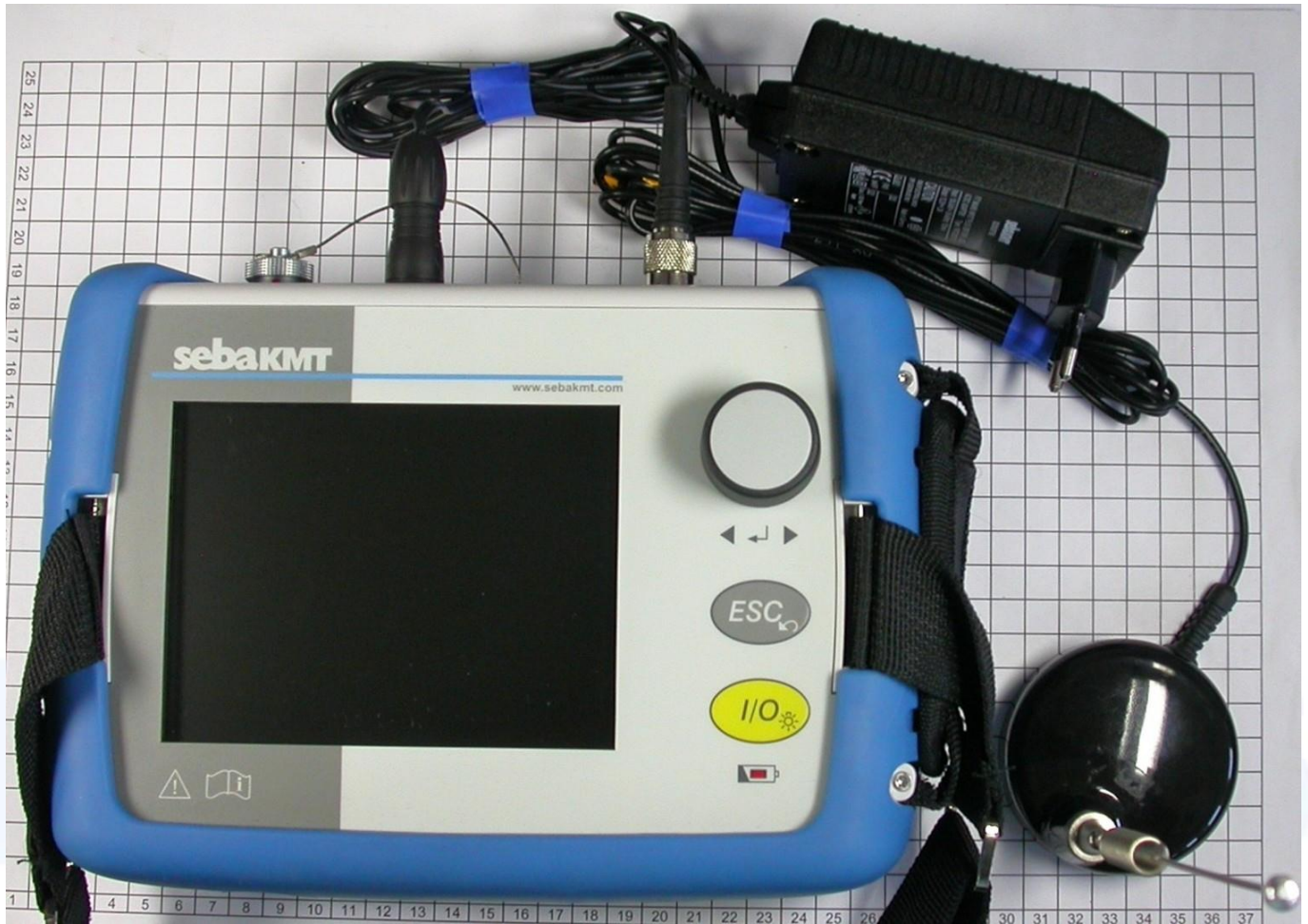
Test setup overview (with AC/DC power supply and magnetic socket antenna)
