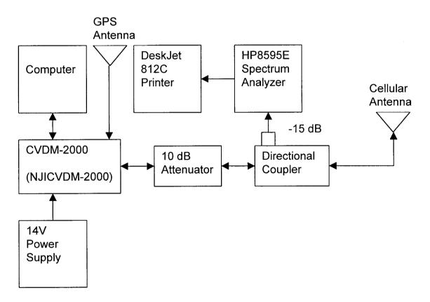
I used a host computer to place an actual call to the UUT (CVDM-2000), established a modem link and then configured the UUT to provide continuous GPS fix information to the host computer (over-the-air). The antenna transmitter output of the UUT was sampled during the data session and the occupied bandwidth plots were made. The plots were hard copies so, I scanned them into my computer and created a PDF file (OccBW.PDF), which I will provide to you as well. The file consists of two pages.
