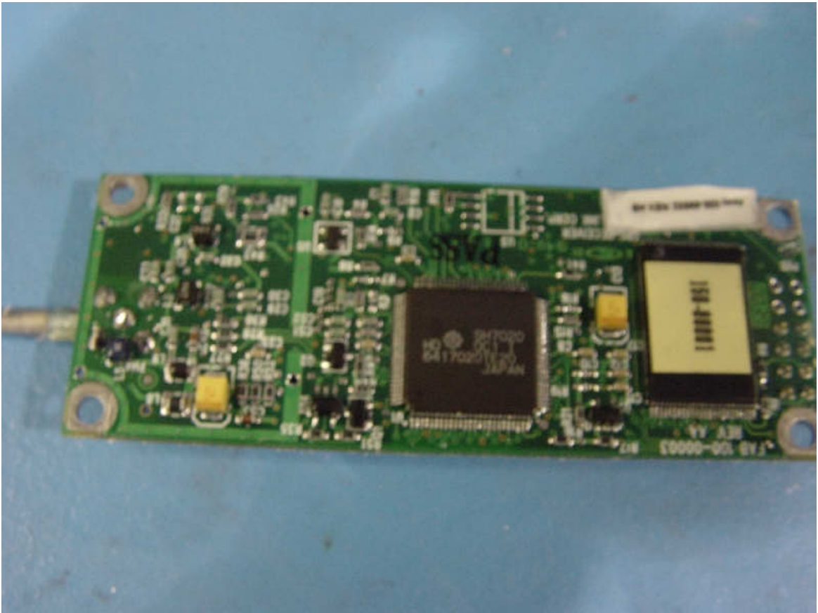
GPS module with RF shield removed (top)
