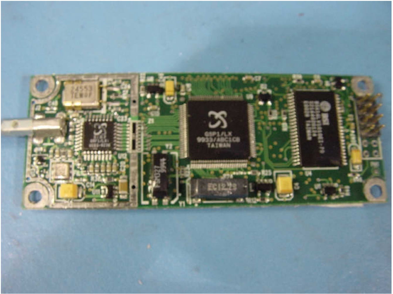
GPS module with RF shield removed (bottom)
