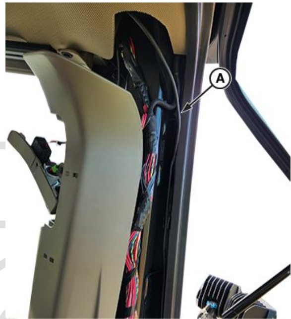
Antenna Cable Routing
