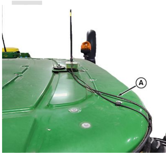
Route Antenna Cable—Cab Roof
