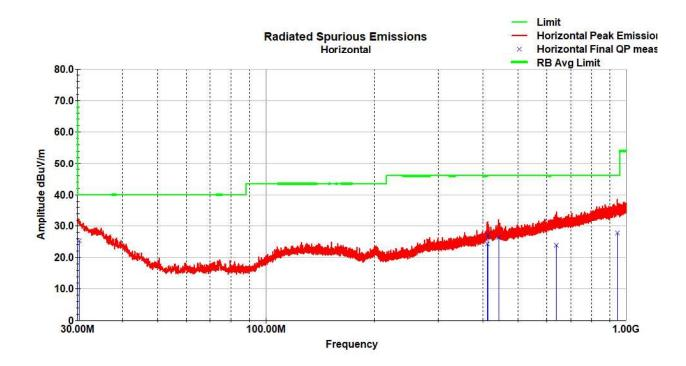
Horizontal Radiated Spurious Emissions Data - 30-1000MHz (802.11g HCH)
