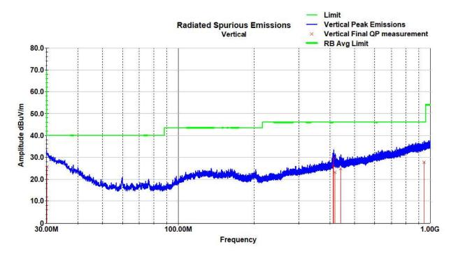
Vertical Radiated Spurious Emissions Data - 30-1000MHz (802.11n LCH)
