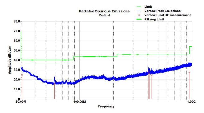
Vertical Radiated Spurious Emissions Data - 30-1000MHz (802.11n MCH)
