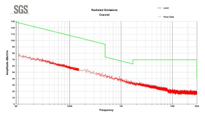
Co-Planar Radiated Spurious Emissions - 9kHz-30MHz (802.11n LCH)
