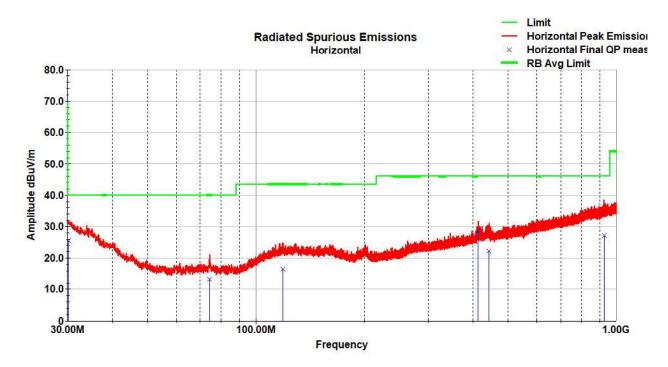
Horizontal Radiated Spurious Emissions Data - 30-1000MHz (802.11n LCH)
