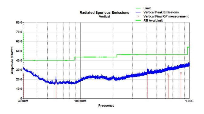
Vertical Radiated Spurious Emissions Data - 30-1000MHz (802.11b MCH)
