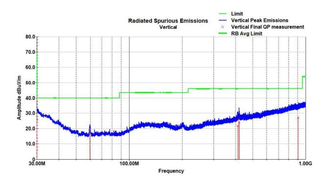
Vertical Radiated Spurious Emissions Data – 30-1000MHz (802.11b HCH)
