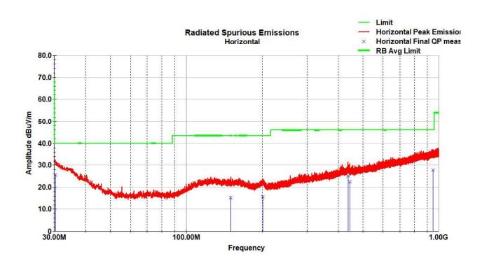
Horizontal Radiated Spurious Emissions Data – 30-1000MHz (802.11b MCH)
