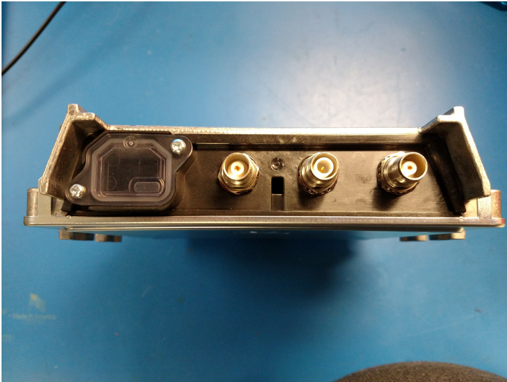
End View - SIM/LED Cover, TNC Cell and GPS Antenna Connectors
