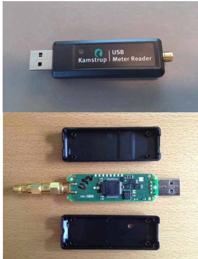
Photo 2.1.1 Exterior (front) and interior stack up of the test object.
