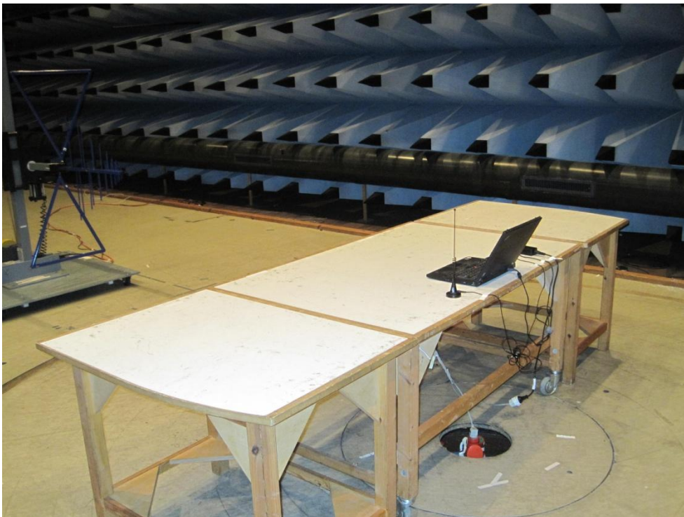
Photo 4.5.2 Test setup regarding measurement radiated limits below 1 GHz.
