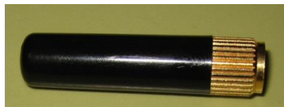
Photo 2.1.2 Antenna option “stubby” used with the test object in one out of two possible configurations.
