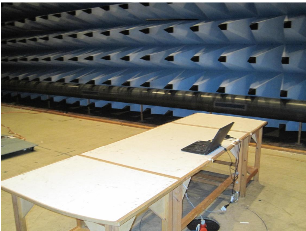
Photo 4.3.2 Test setup regarding measurement radiated limits below 1 GHz.
