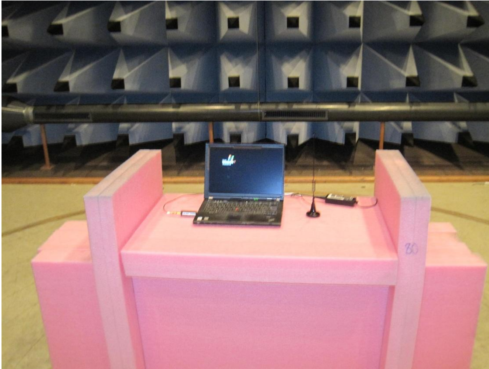
Photo 4.6.1 Test setup regarding measurement radiated limits above 1 GHz.
