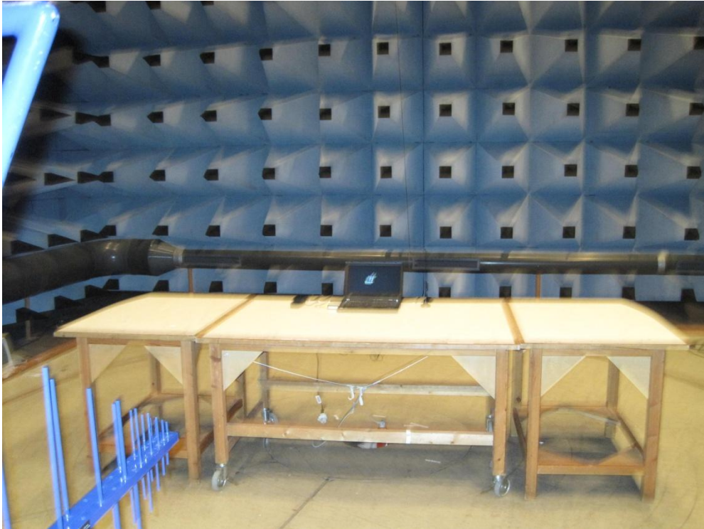
Photo 4.3.1 Test setup regarding measurement radiated limits below 1 GHz.
