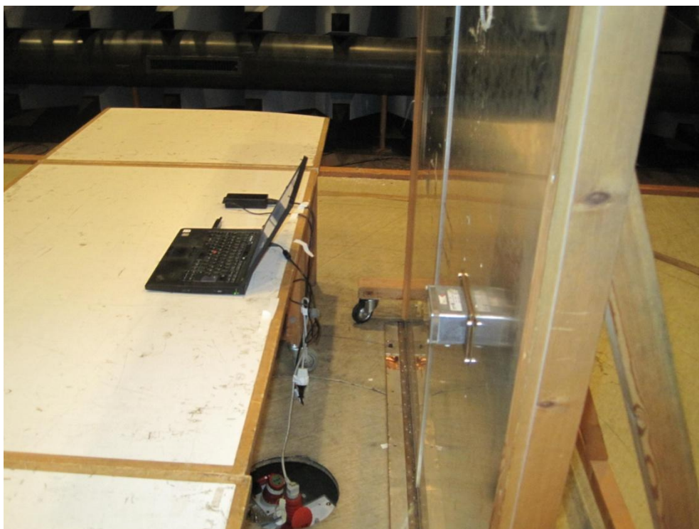
Photo 4.1.2 Test setup regarding measurement of conducted limits, AC Mains.
