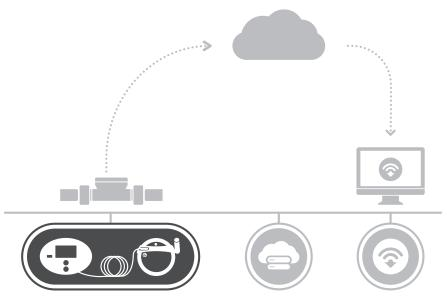
READy MTU connects to an encoded output meter and sends data to READy Collector and READy Manager.
