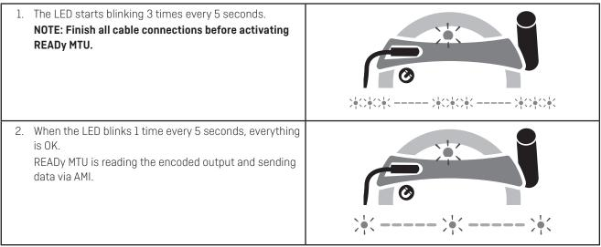
The LED automatically stops blinking after 5 minutes. No further configuration is needed.
