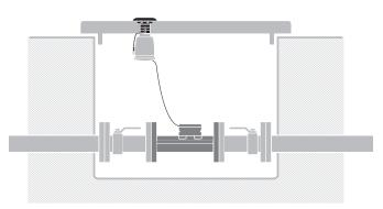
You can use the pit antenna or the wall bracket with a rebar or similar to install READy MTU in pits.
