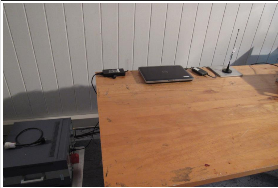
Conducted test setup with roof top antenna
