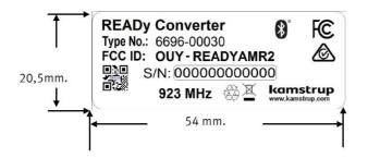
No. of digits in Type No.: 9 No. of digits in Serial No.: 8 ( Scanned from PCB))
