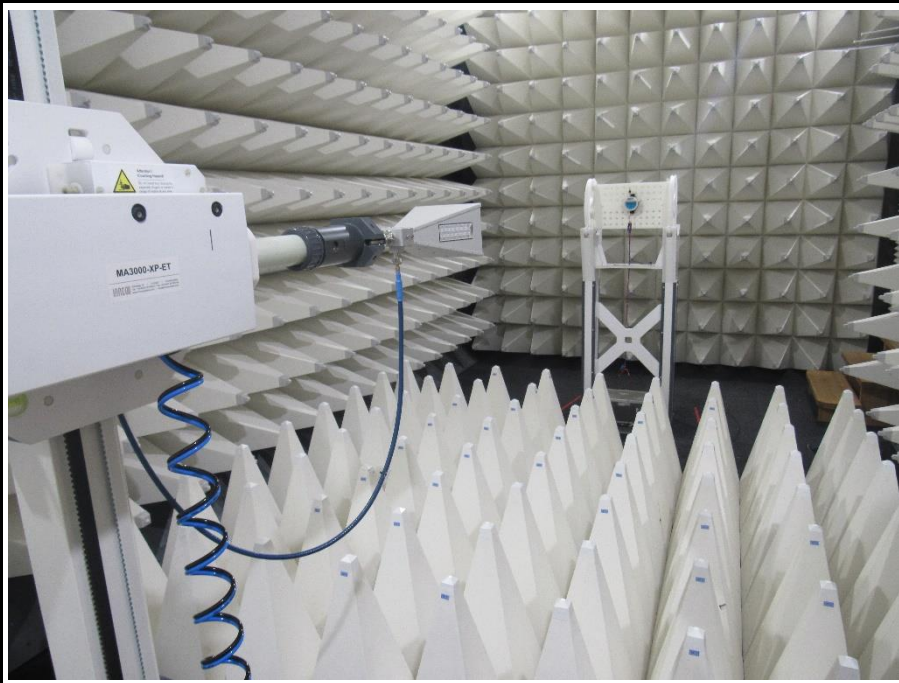
Setup for measurements above 1 GHz
