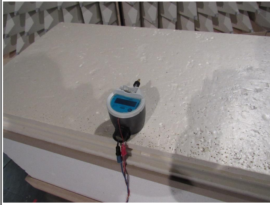
Test Setup with 10 dB attenuator and 50 Ohm load
