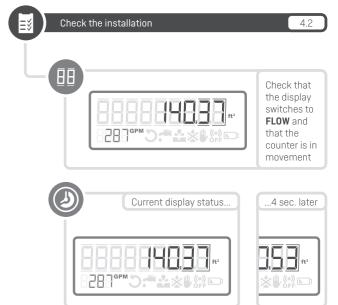
The first 8 hours the meter operates in Installation Mode. The display will update every 4 seconds during Installation Mode, permitting the installer to confirm that the meter is properly operating. Every time the meter becomes dry and subsequently rewetted, Installation Mode will re-initiate
