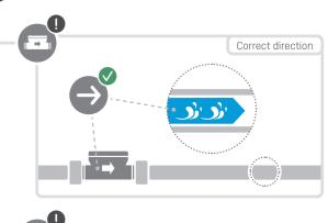
Install meter in the correct direction of flow
