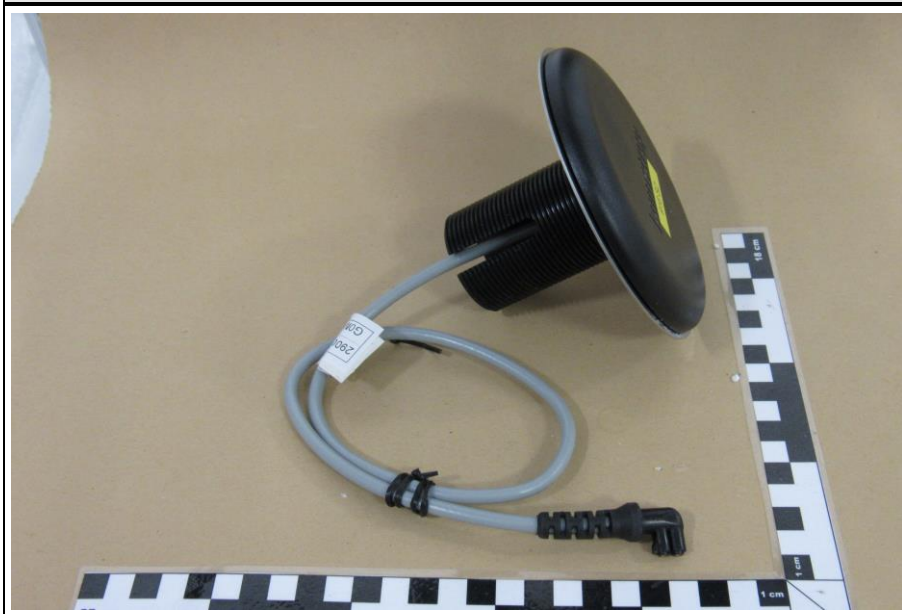
External Antenna Side View
