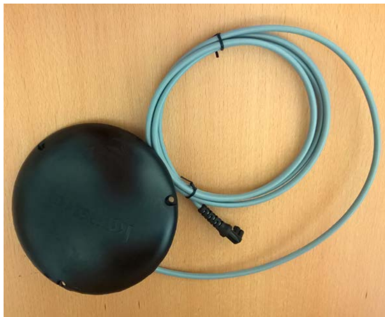
Kamstrup antenna and proprietary connector
