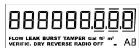
When flowIQ® 2100 leaves Kamstrup Headquarters, it has been tested and verified and the counter has been reset. The number of gallons or CuFt are displayed by nine large digits (Bars over and under digits indicates decimals after the comma). A number of info codes can be displayed, of which 'DRY' and 'RADIO OFF' will be activated and flash upon delivery. Furthermore, the small square in the bottom right-hand corner flashes to indicate that the meter is active.
