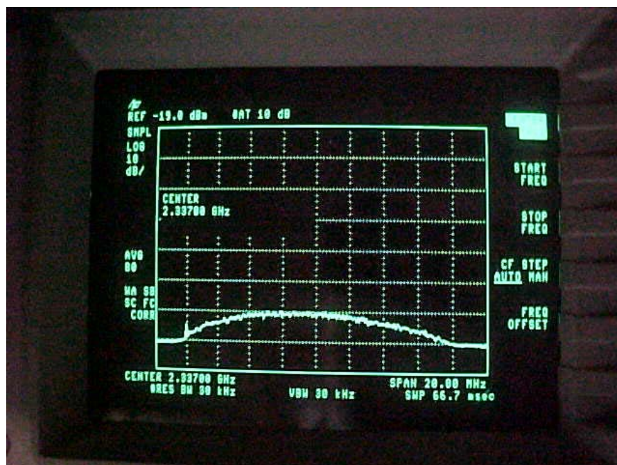
Figure 4-8C. Third Harmonic (2337.00 MHz) = -79.0 dBm (Pre-Filter)
