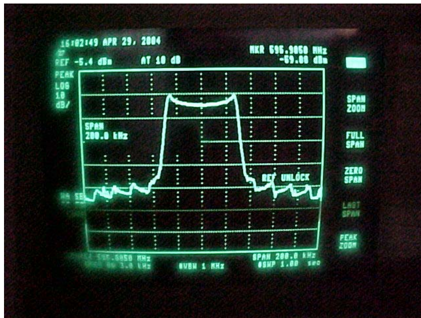
Figure 4-8. Aural Carrier Occupied Bandwidth
