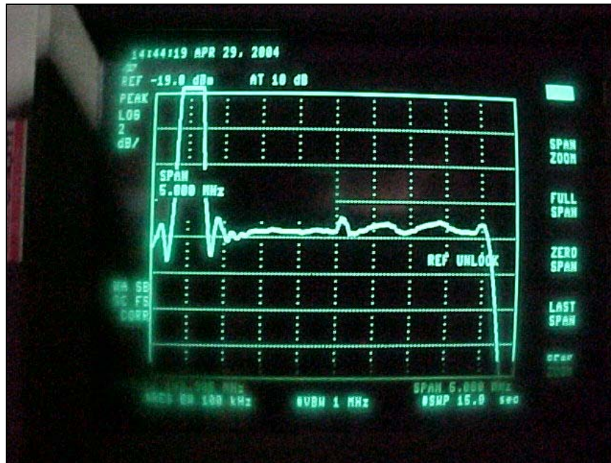
Figure 4-3. Graph of Detected Video Frequency Response
