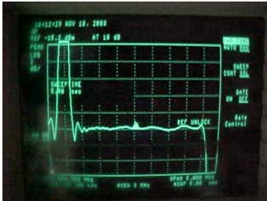
Figure 4-3. Graph of Detected Video Frequency Response
