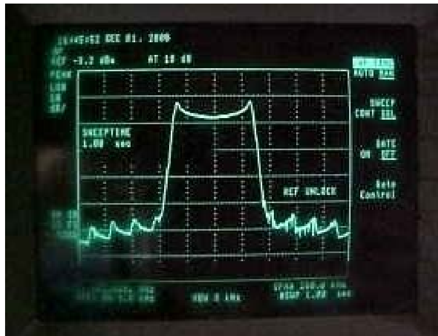
Figure 4-8. Aural Carrier Occupied Bandwidth
