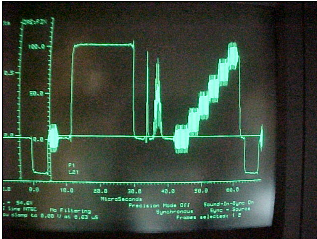
Figure 4-2. Substantially Linear Transfer Characteristics of the Transmitter as a Demodulated Video Waveform
