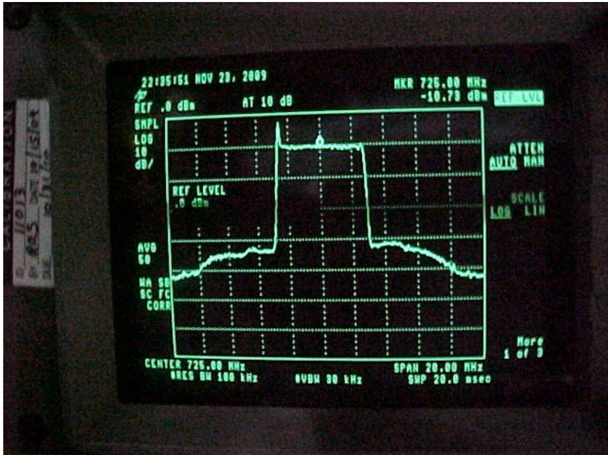
Echostar 5 5kW HXB spectrum Ch56 occupied BW
