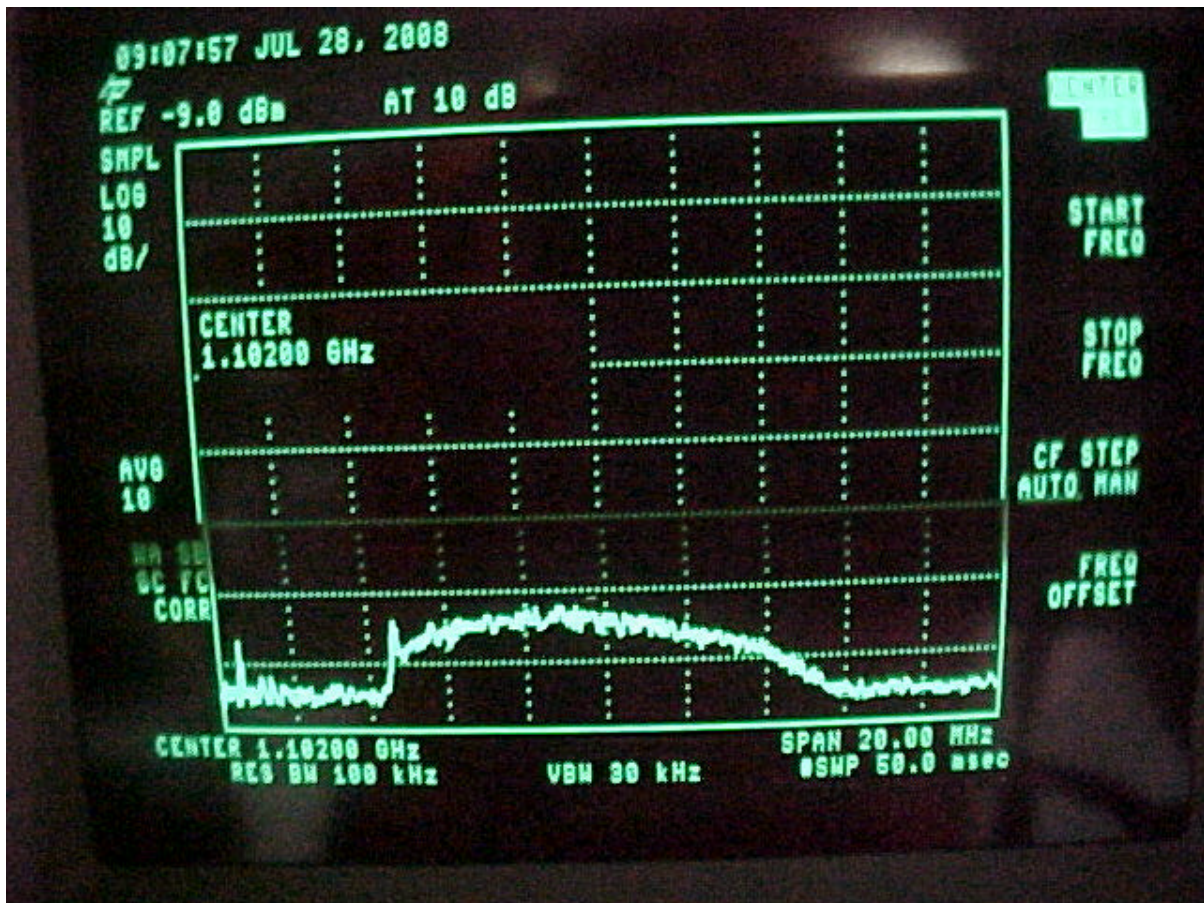
Figure 4-8B. Second Harmonic 1102 MHz) = -71 dBm (Pre-Filter)
