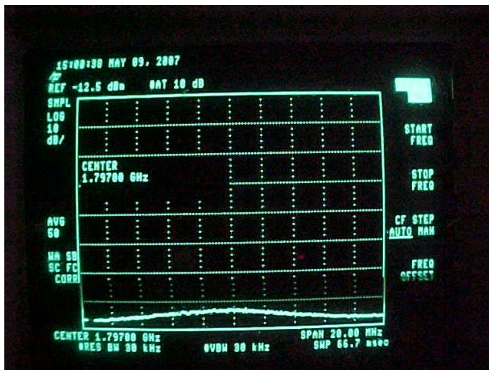
Figure 4-8C. Third Harmonic (1797 MHz) = -85.50 dBm (Pre-Filter)
