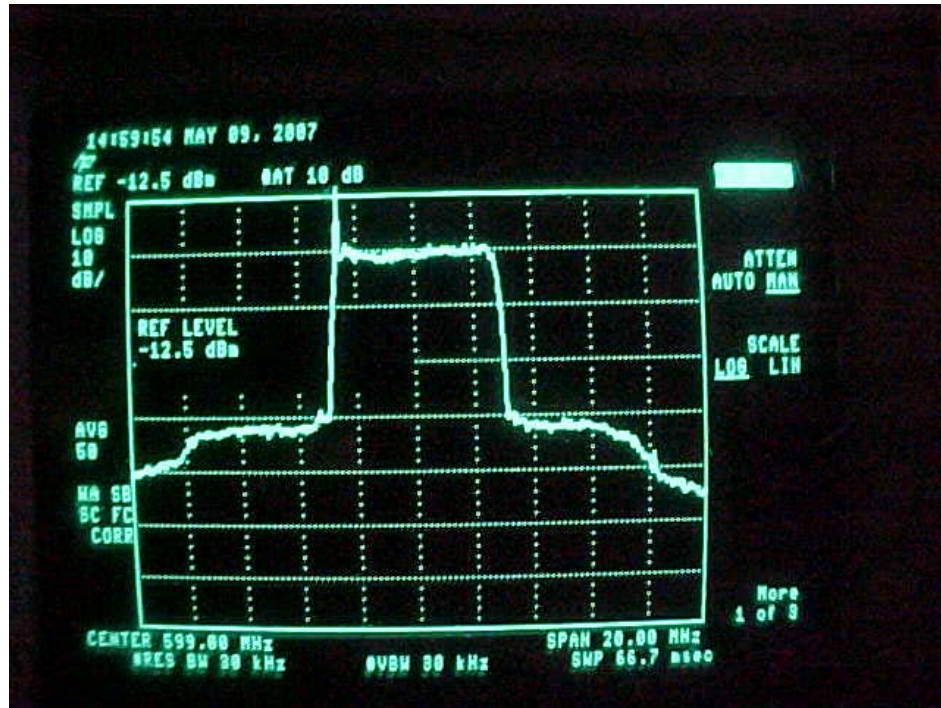
Figure 4-8A. Reference (599 MHz) = -12.50 dBm (Pre-Filter)
