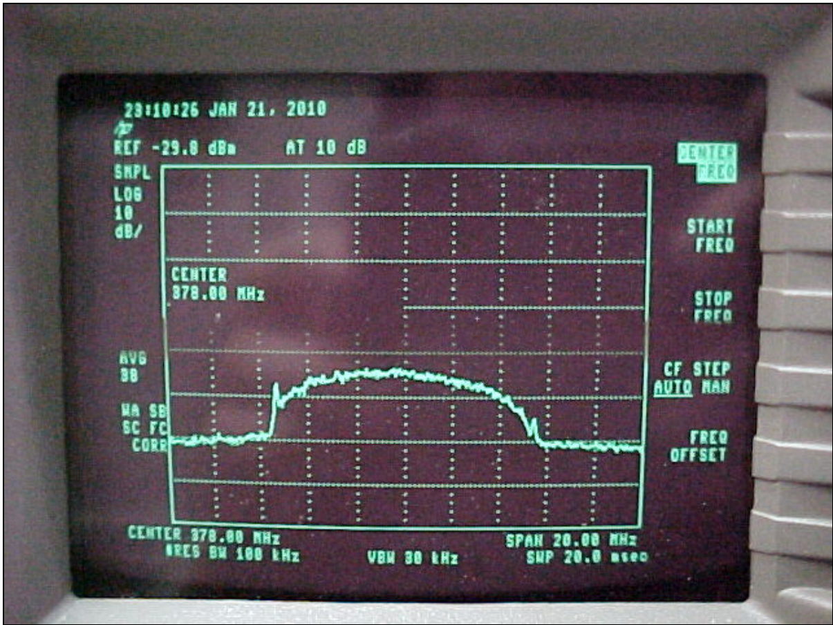
Figure 4-8C Second Harmonic (Pre-Filter)
