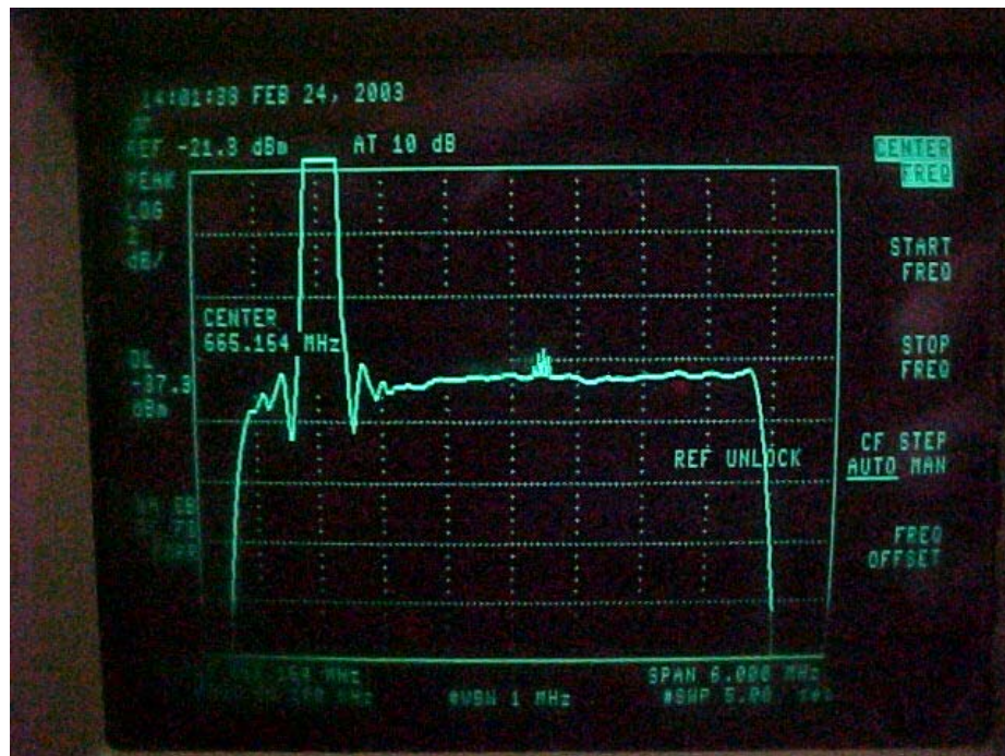
Figure 4-3. Graph of Detected Video Frequency Response
