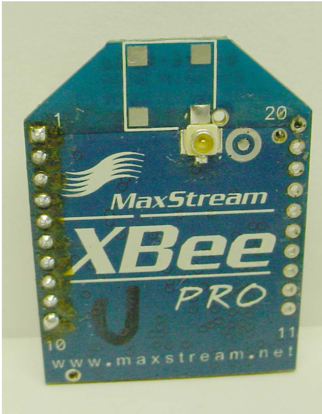
EUT with U.FL connector
