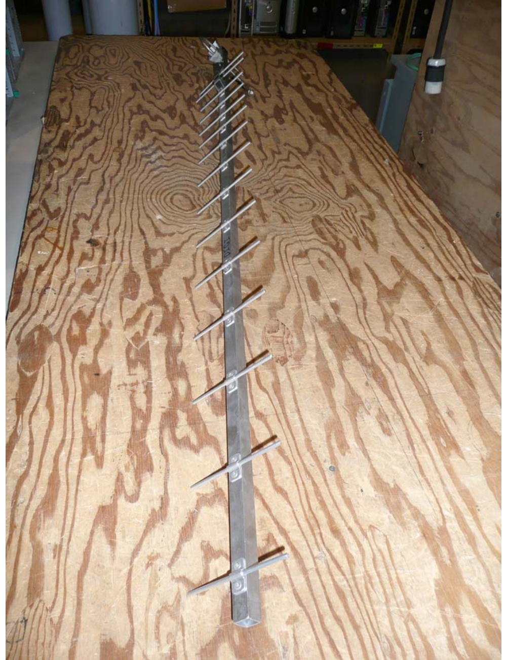
A09-Y15TM, 15 Element Yagi Antenna, 15.1 dBi gain
