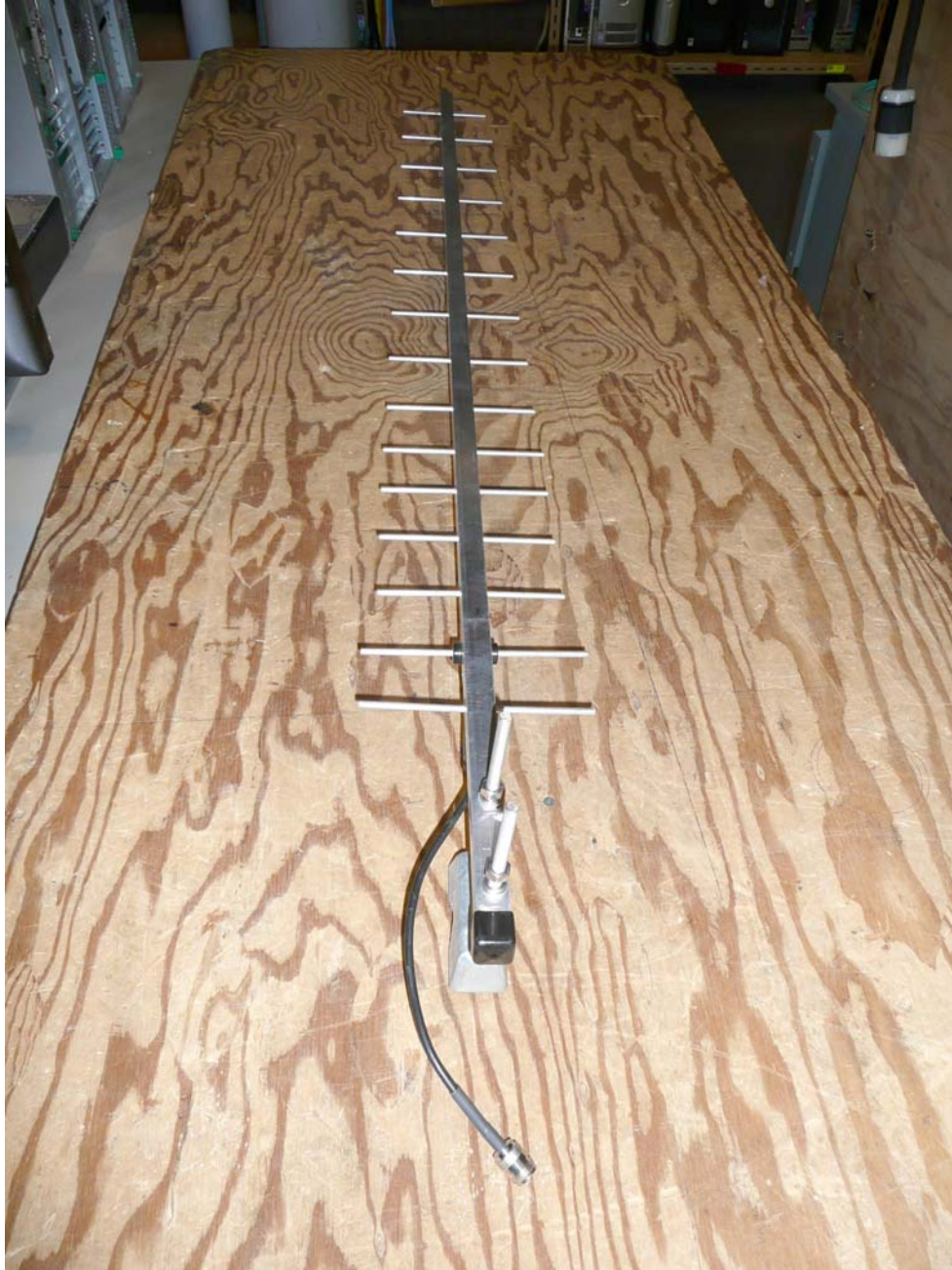
A09-Y15TM, 15 Element Yagi Antenna, 15.1 dBi gain
