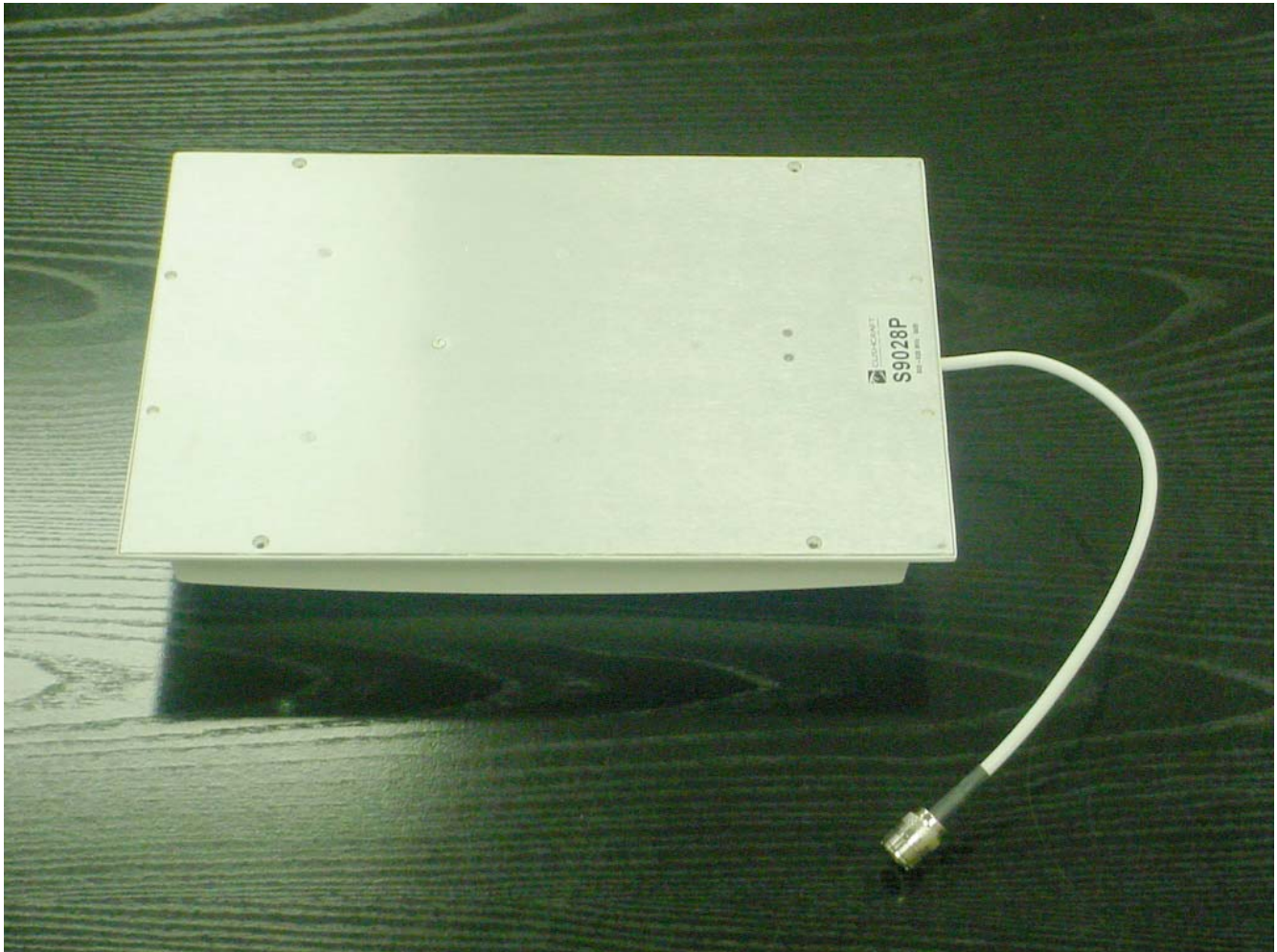
Panel Antenna (A09-P8TM, 8dBi Panel antenna, RPTNC)
