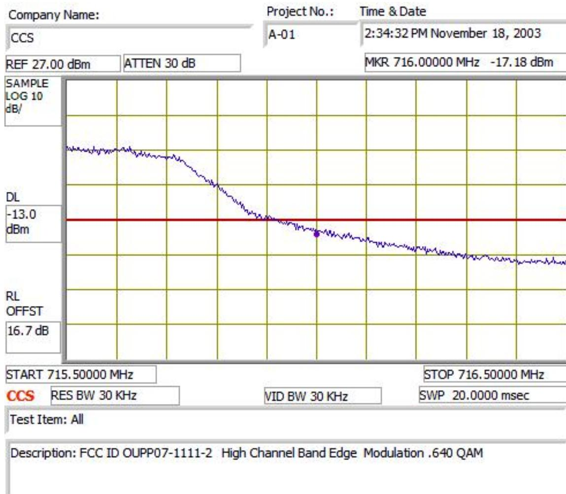
High Channel, 16QAM 640 ksym/sec, fc = 715.4 MHz
