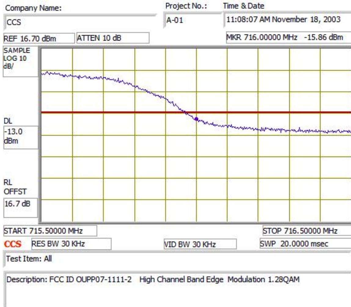
High Channel, 16QAM 1280 ksym/sec, fc = 715.1 MHz
