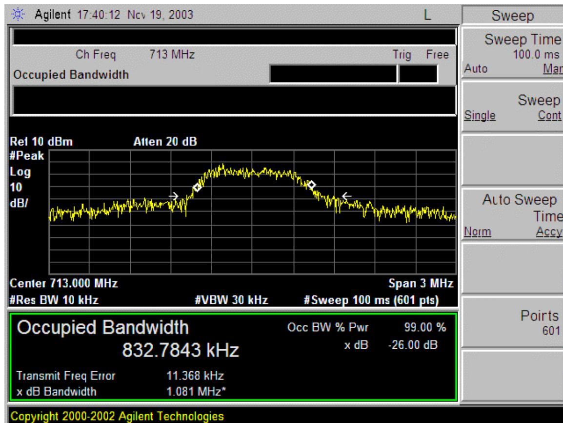
Occupied Bandwidth, 1280 ksym/sec, 16QAM
