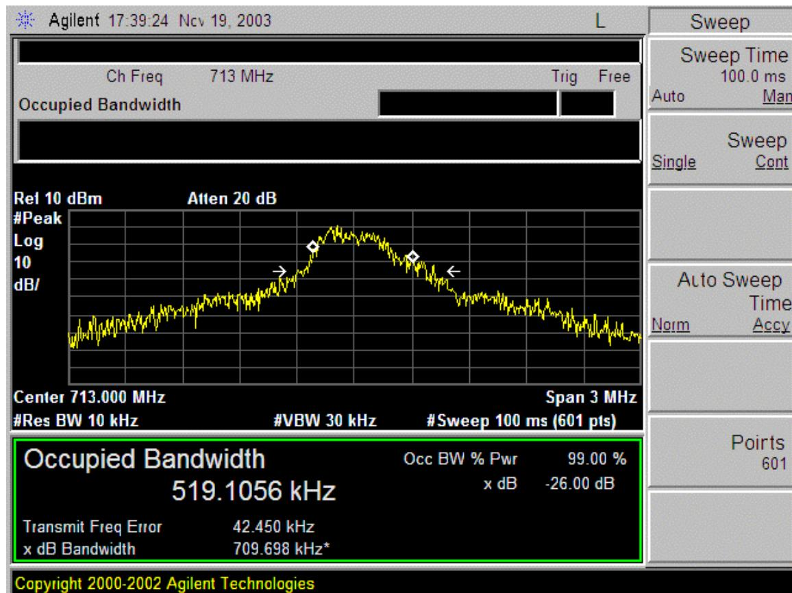
Occupied Bandwidth, 640 ksym/sec, 16QAM
