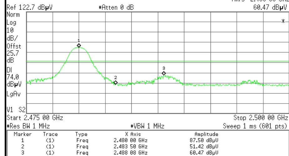
**Detector mode : Average****Polarity : Vertical****CH High****Agilent 23:36:12 Oct 29, 2007****Mkr3 2.483 96 GHz
