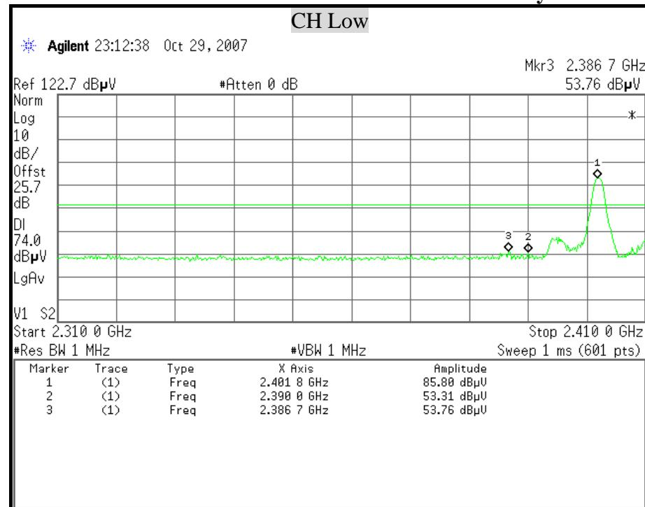
**Detector mode : Average****Polarity : Vertical**
