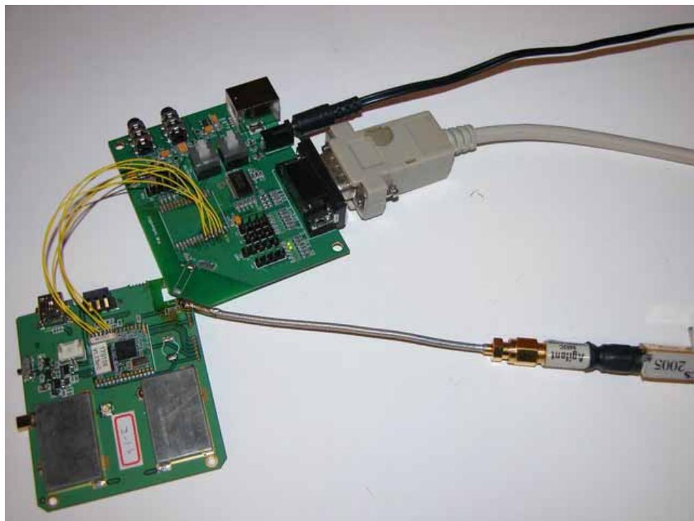
**POWERLINE CONDUCTED EMISSIONS MEASUREMENT SETUP****FOR 120VAC/60Hz**
