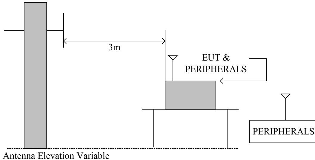
The diagram below shows the test setup that is utilized to make the measurements for emission above 1GHz.
