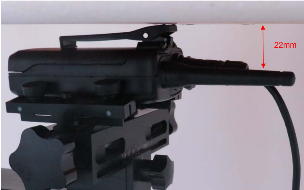
Picture 4: Body-worn, the front of the EUT towards ground, Belt clip directed tightly to touch the bottom of the flat phantom, the distance from the EUT Antenna to the bottom of the Phantom is 22mm
